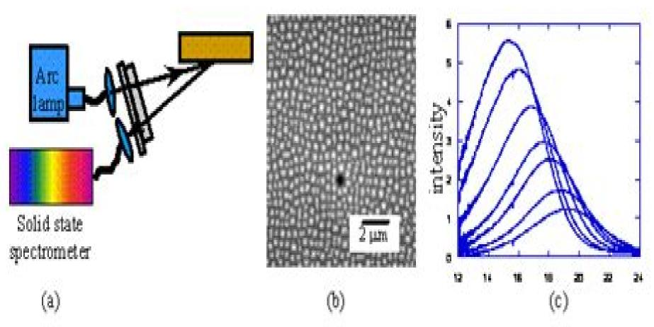
Figure 3. Light scattering spectroscopy measures surface PSD optically at fixed scattering angles. (a) The scattered intensity is measured as a function of wavelength. (b) An AFM image of an array of quantum dot islands (c) The corresponding light scattering from an island array as it evolves during growth.
