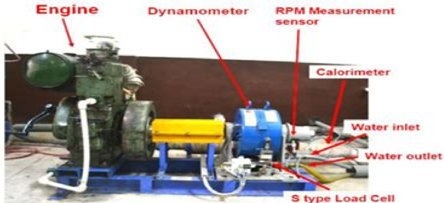
Plate 1. Engine with eddy current dynamometer
