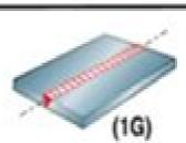
Plates and axis of pipe horizontal
