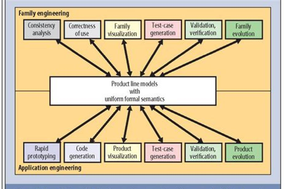
Figure 1. A model-centric development process for software product lines based on a uniform formal modeling framework can evolve into a single-source technology that offers several important advantages over the current state of the art in SPLE.
