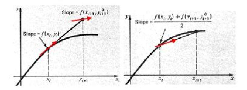
$$y^{0}(x + \Delta x) = y(x) + f(x, y(x))\Delta x \qquad \text{(Predictor)}$$
