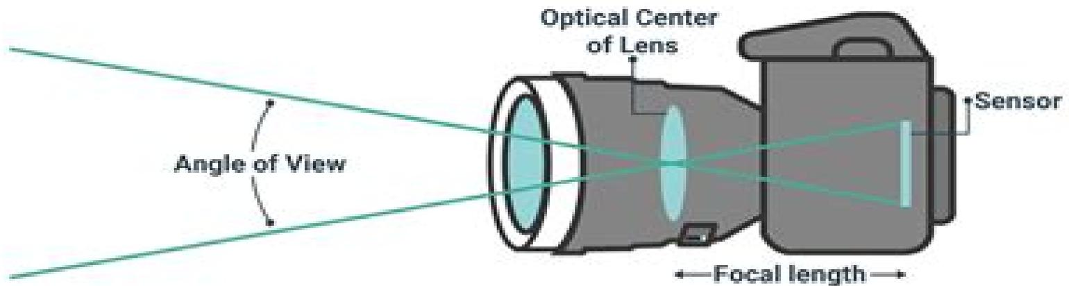
Focal Length is the distance between the optical center of a lens and the camera image sensor
