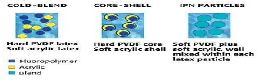
Figure 2/Expected resin morphology in film, based on three latex morphology cases.
