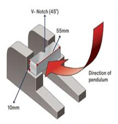
The Charpy impact test, also known as the Charpy V-notch test, measures the energy absorbed by a material when fractured under impact. A pendulum strikes a notched specimen (55 mm long, 10 mm square, with a 2 mm deep V-notch), and the energy is recorded in joules.
