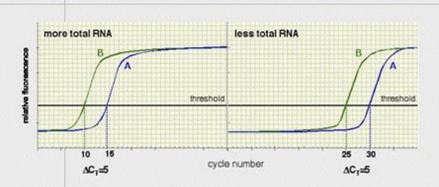
When the PCR efficiency of both systems is the same the  $\Delta C_T$  remains constant
