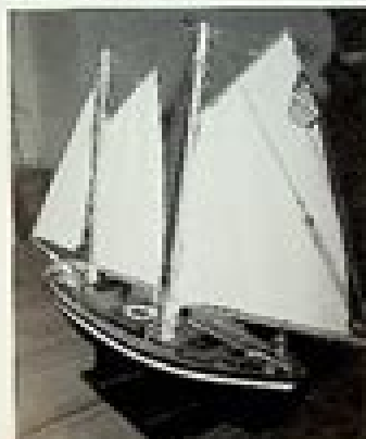
Fig. 4.17 American pinkie, a schooner-rigged model of the Light 1820
