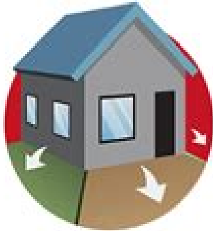
PROPERLY GRADED YARD
