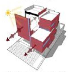
THE GLASSLESS FACADE CONCEPT WAS DESIGNED TO PREVENT THE SOUND LEARS FROM THE INSIDE TO THE OUTSIDE AND VICE YERSA. IT WAS ALSO MEANT TO PREVENT THE MAXIMUM SUN RADIATION FROM THE WEST.
