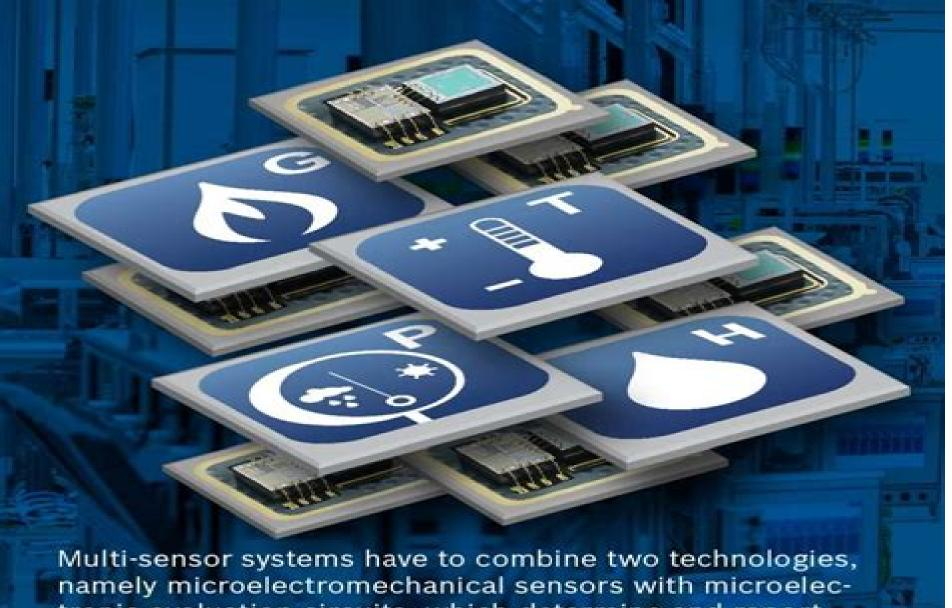
Multi-sensor systems have to combine two technologies, namely microelectromechanical sensors with microelectronic evaluation circuits, which determine and report such things as temperature, light intensity, chemical concentrations, and humidity.
