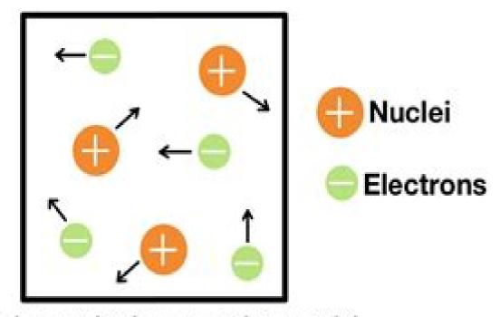
Particles are broken apart into nuclei and electrons due to high heat. These broken apart particles act similarly to gas particles, moving freely with no distinct arrangement
