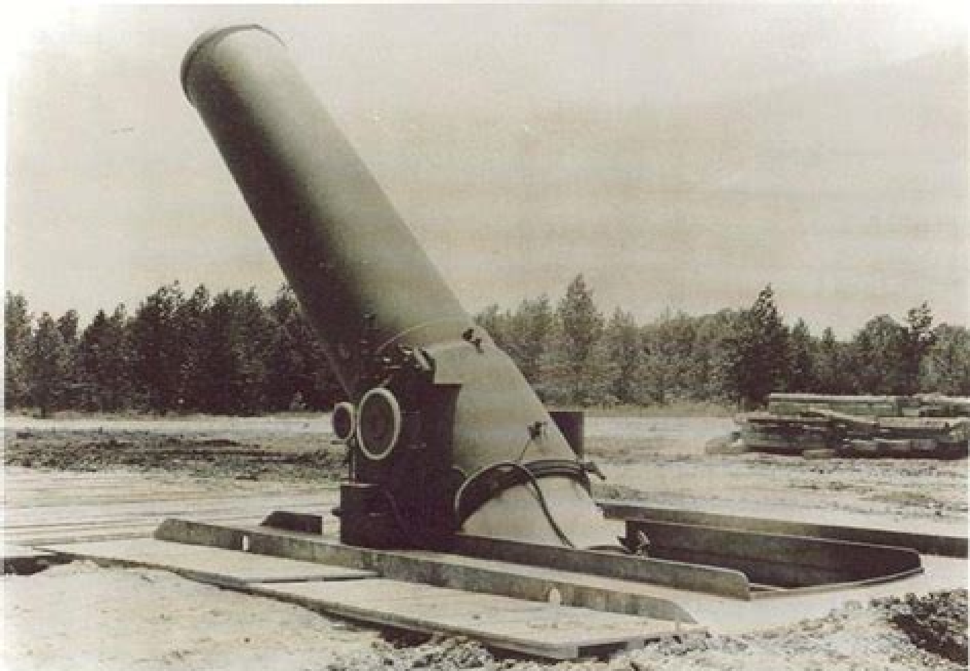
U.S. "LITTLE DAVID" 914MM(36 INCH) MORTAR BIGGEST MORTAR IN THE WORLD, CIRCA 1944
