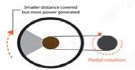
Low gear On a bicycle, a lower gear converts pedal rotation into more power for climbing hills, at the cost of speed
